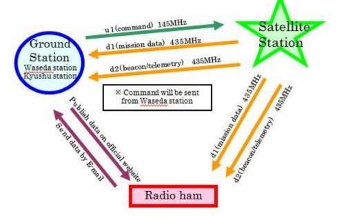
Fig. Overview of communication subsystem
